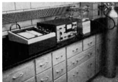
Fig. 5.—Equipment employed for measuring resistivity as a function of temperature.
